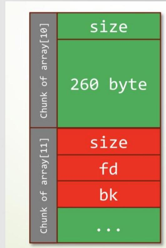
memcpy() lead to heap overflow
