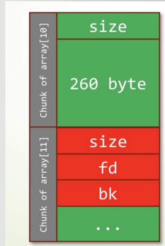
memcpy() lead to heap overflow
