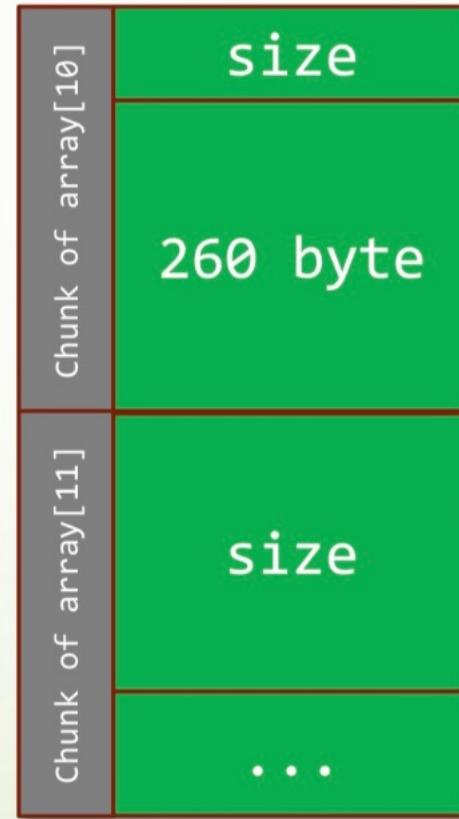
memcpy() lead to heap overflow
