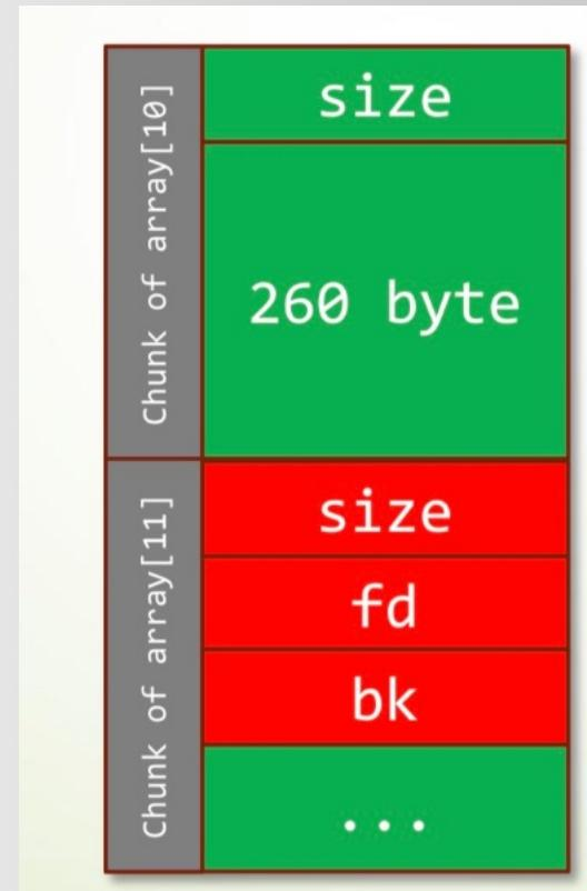
memcpy() lead to heap overflow
