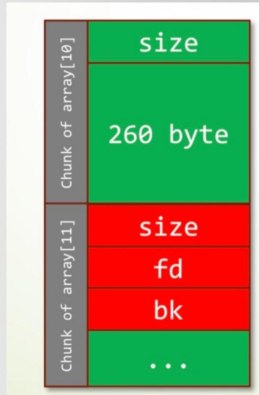
memcpy() lead to heap overflow
